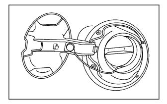
The tethered fuel cap is located behind a hinged fuel door on the driver's side of the vehicle. If the vehicle has E85 fuel capability, a yellow cap with the words "E85/gasoline" can be seen.
